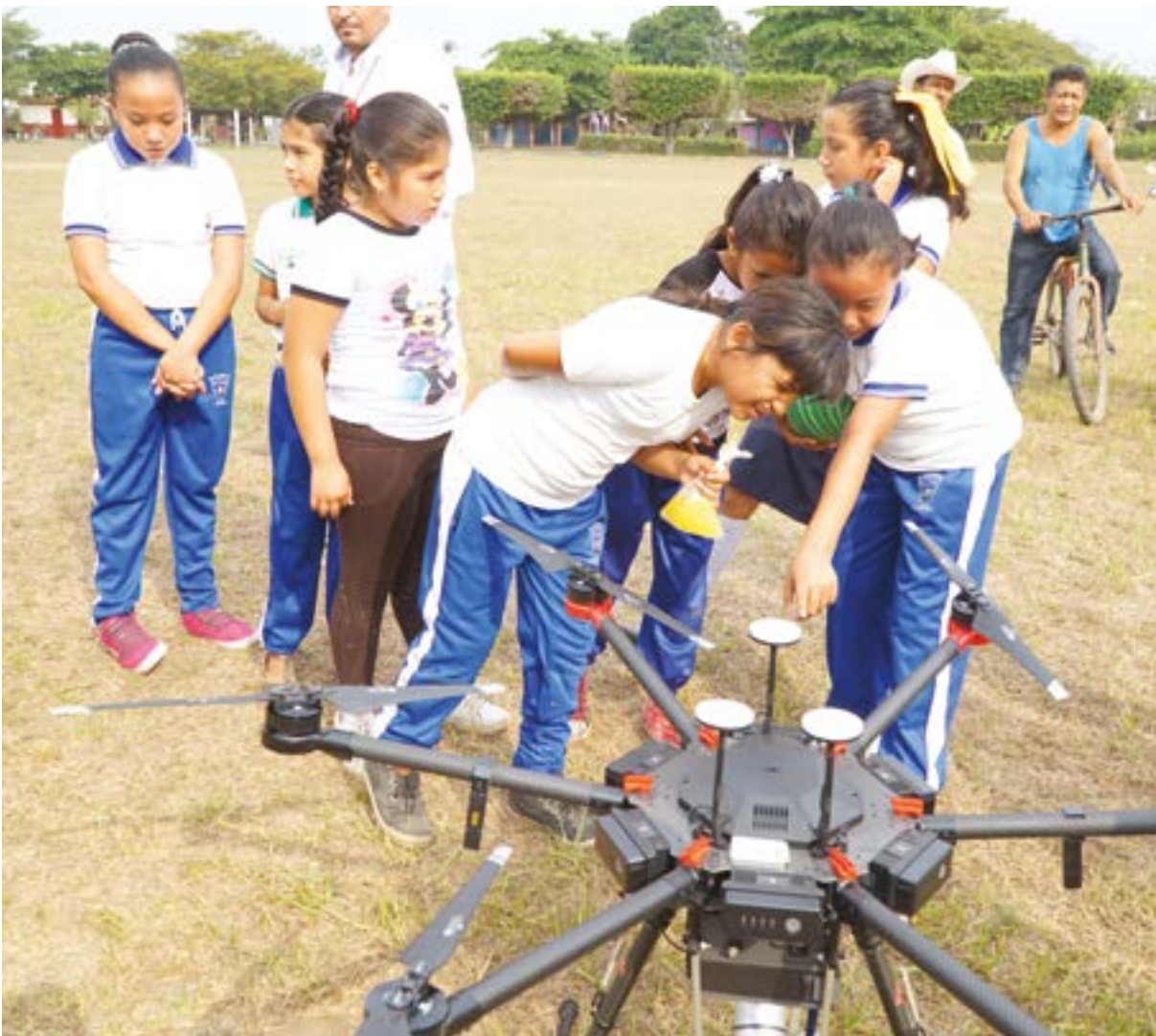
This drone releases sterile male mosquitoes to help reduce transmission of dengue, Zika and Chikungunya.
